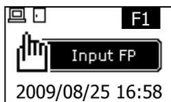
When you place the finger on the fingerprint sensor, the fingerprint input window is lighted in red along with "ppik" sound. Leave the finger until the light is switched off.
